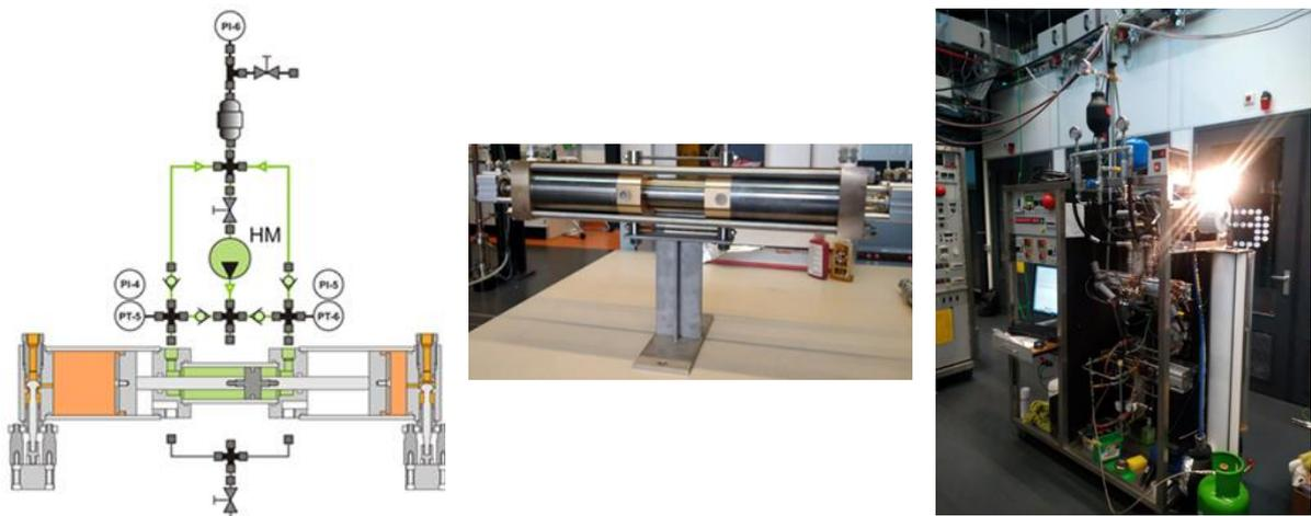
Figure 46 Experimental Worthington-type IEE coupled with hydraulic motor, HM, its picture and picture of the test rig
