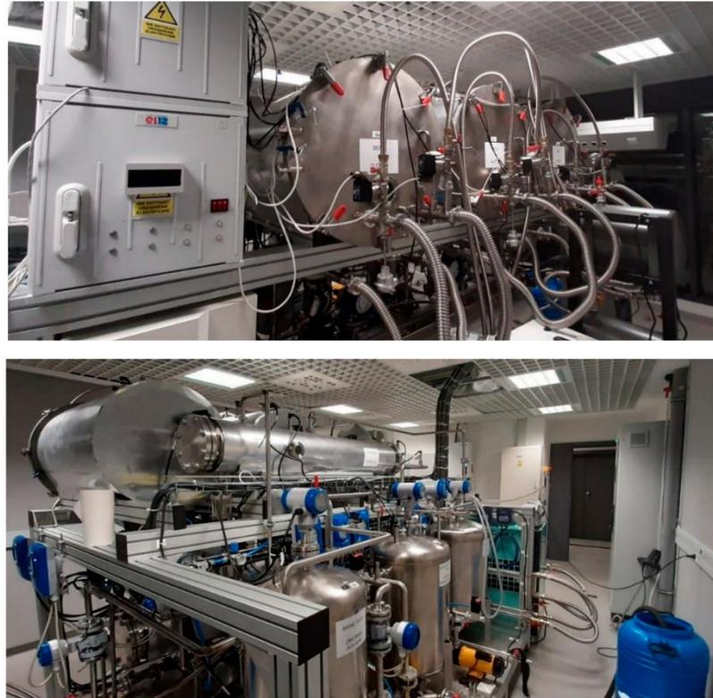
Figure 24 Experimental prototype of a three-bed hybrid chilling (1.1 kW) and desalination adsorption device, front view (top picture) and back view (bottom picture) [44]
