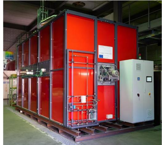
Figure 33 Lumenion steel-based thermal energy storage, left: conceptual design, right: actual 450 kWh implementation in University of Applied Sciences (HTW) laboratory [91]
