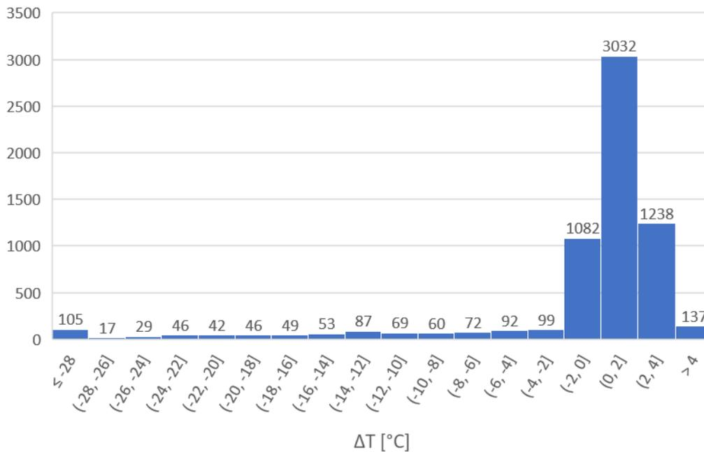
Figure 24: Variation of main engine exhaust gas temperature histogram due to the operation of the eSAILs along selected example trading routes based on 2017-2021 historical wind data.
