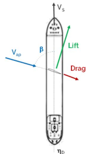
Figure 11: eSAIL loads on a vessel
