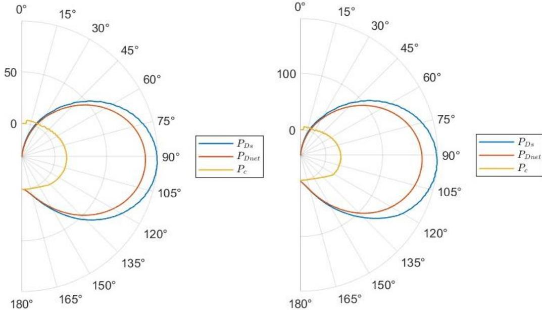
Figure 15:  $P_{Dnet}$ ,  $P_{Ds}$  and  $P_c$  [in kW] for (2x) 17x2.85m eSAIL at  $V_s=11.8\text{knot}$  at  $V_T=10\text{kn}$  (left) and  $V_T=14\text{kn}$  (right), plotted wrt True Wind Angle (TWA)
