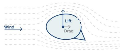
Figure 4: eSAIL aerodynamic behavior with suction ON
