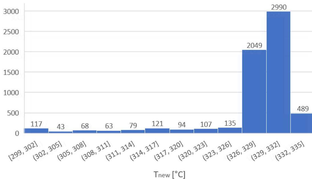
Figure 23: Resulting main engine exhaust gas temperature histogram due to the operation of the eSAILs along selected example trading routes based on 2017-2021 historical wind data.
