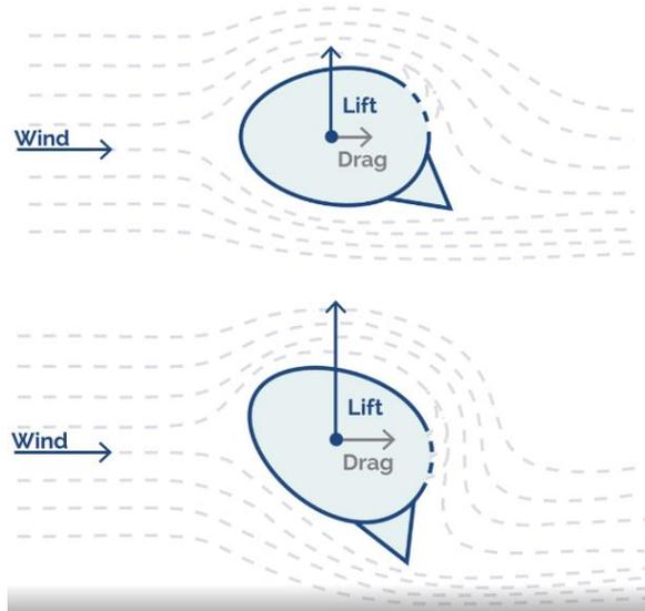
Figure 7: eSAIL in operation (suction on), at two different angles of attack
