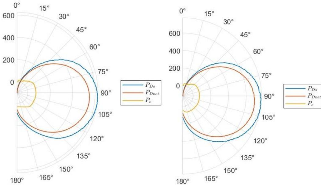
Figure 17:  $P_{Dnet}$ ,  $P_{Ds}$  and  $P_c$  [in kW] for (2x) 17x2.85m eSAIL at  $V_s=11.8$ knot at  $V_T=26$ kn (left) and  $V_T=30$ kn (right), plotted wrt True Wind Angle (TWA)
