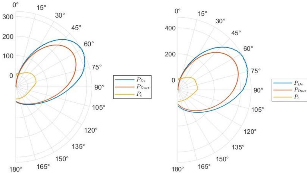
Figure 19:  $P_{Dnet}$ ,  $P_{Ds}$  and  $P_c$  [in kW] for (2x) 17x2.85m eSAIL at  $V_s=10$ knot at  $V_T=18$ kn (left) and  $V_T=22$ kn (right), plotted wrt Apparent Wind Angle (AWA)
