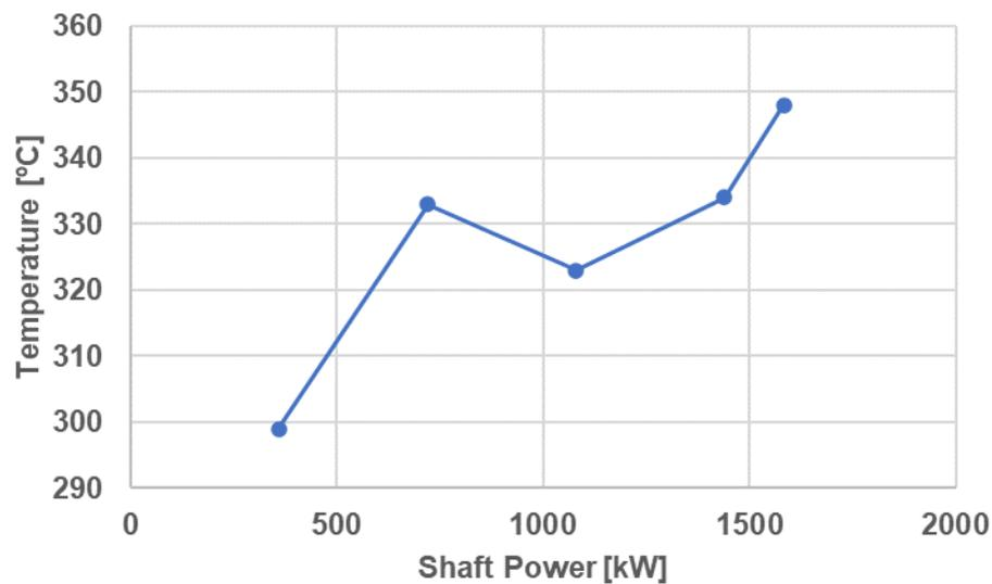
Figure 14: Eems Traveller main engine exhaust gas temperature depending on engine power.
