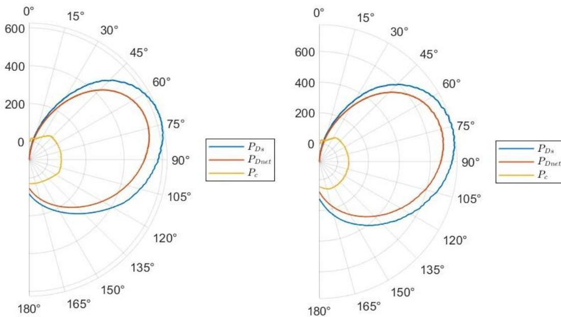
Figure 20:  $P_{Dnet}$ ,  $P_{Ds}$  and  $P_c$  [in kW] for (2x) 17x2.85m eSAIL at  $V_s=10$ knot at  $V_T=26$ kn (left) and  $V_T=30$ kn (right), plotted wrt Apparent Wind Angle (AWA)
