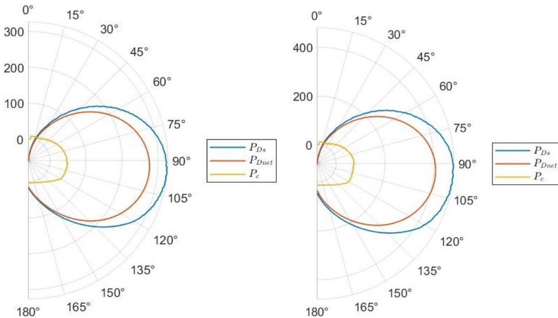
Figure 16:  $P_{Dnet}$ ,  $P_{Ds}$  and  $P_c$  [in kW] for (2x) 17x2.85m eSAIL at  $V_s=11.8\text{knot}$  at  $V_T=18\text{kn}$  (left) and  $V_T=22\text{kn}$  (right), plotted wrt True Wind Angle (TWA)
