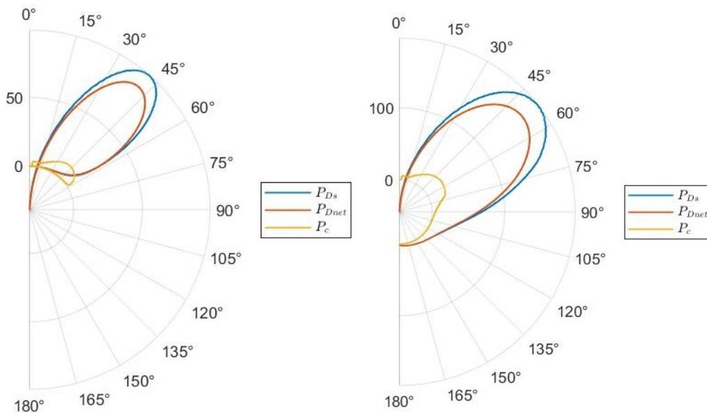
Figure 18:  $P_{Dnet}$ ,  $P_{Ds}$  and  $P_c$  [in kW] for (2x) 17x2.85m eSAIL at  $V_s=11.8$ knot at  $V_T=10$ kn (left) and  $V_T=14$ kn (right), plotted wrt Apparent Wind Angle (AWA)
