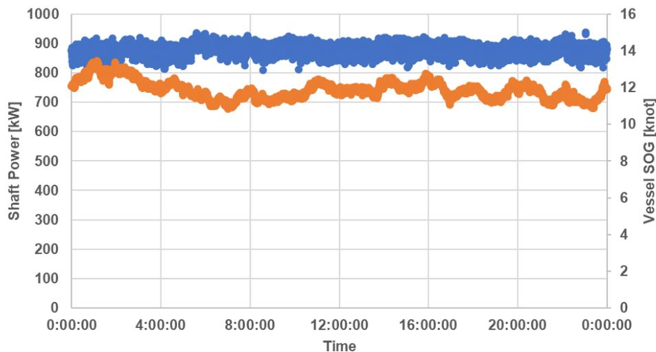
Figure 12: Eems Traveller sailing speed vs. shaft power
