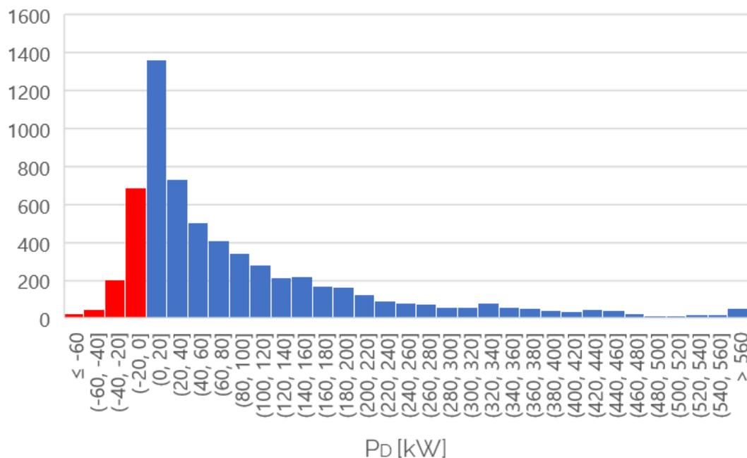
Figure 22: eSAILS engine-equivalent power savings histogram along selected example trading routes based on 2017-2021 historical wind data
