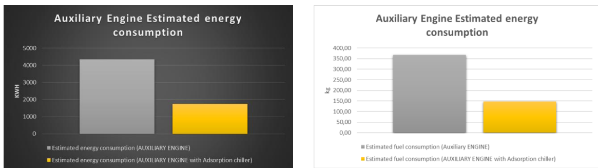
Figure 13: Energy and fuel consumption of auxiliary engine.
