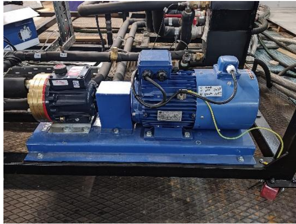
Figure 19 – Photograph of the working fluid pump and motor installed on the ORC–ejector integrated heat pump prototype.
