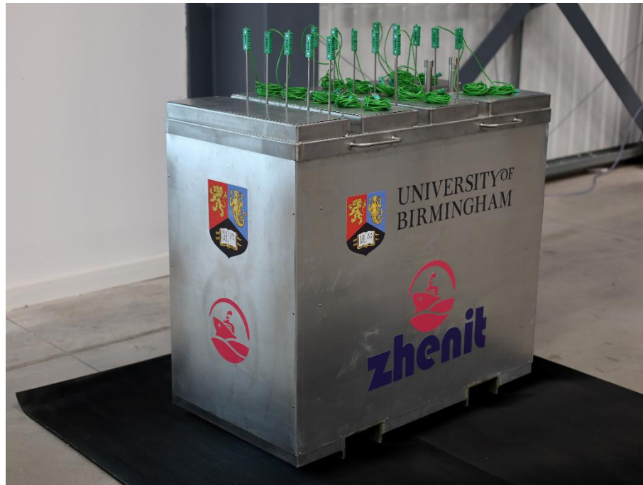
Figure 1 – Photograph of the latent heat thermal energy storage prototype developed by The University of Birmingham .
