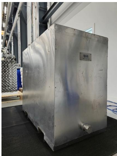
Figure 4 – Photographs of the thermally insulated tank: (left) isometric view and (right) side view.
