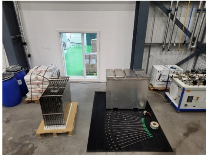
Figure 3 – Photograph of the thermally insulated tank and lid, the drain valve with washer, the bundle of pillow plates with the spacers, the PCM, and the thermocouples with the dedicated wire and compression fittings.
