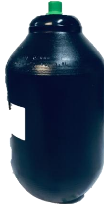
Figure 29 – Photograph of the high-pressure accumulator H4000R utilised in the IEE prototype.
