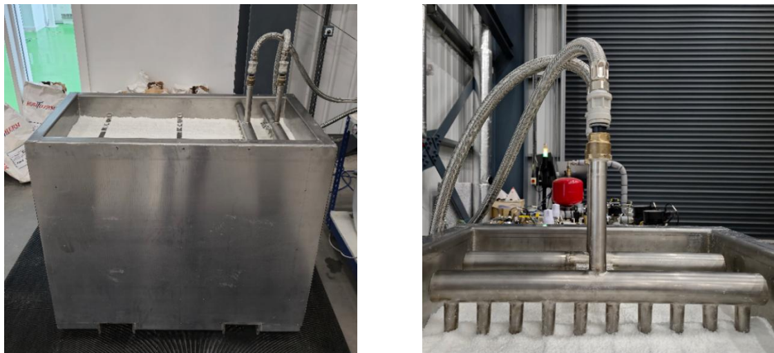
Figure 10 – Photographs of the tank containing the phase change material RT80HC and the pillow plate bundle: (left) side view and (right) close-up of the pipes, manifold, and storage medium.
