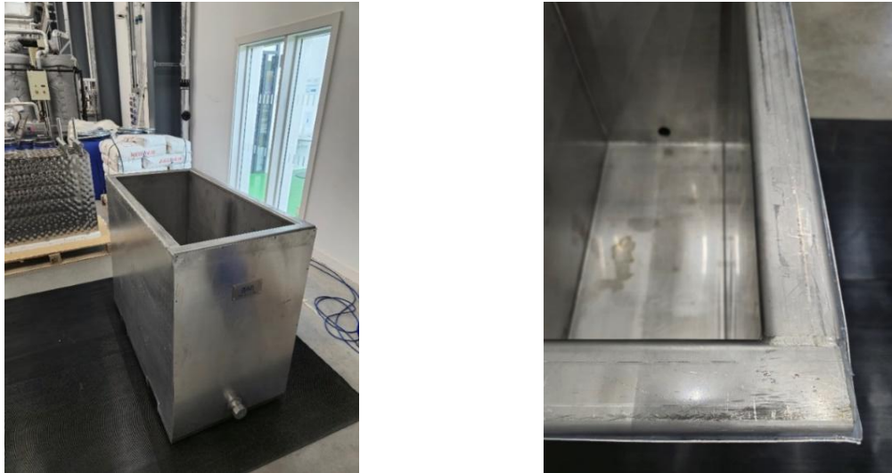
Figure 5 – Photographs of the thermal insulation, aluminium cladding, and heat-resistant silicone of the tank: (left) isometric view and (right) close-up of the side walls.
